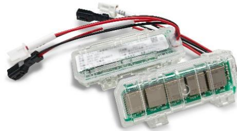
Maxell's all-solid-state battery power module
